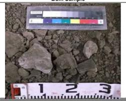
Sample consists of muddy limestone & sandy limestone with fine grained grey/brown coatings. No mineralogical changes, encrustations (e.g. gypsum) or calcareous mudstone. Sample in a dry state.
